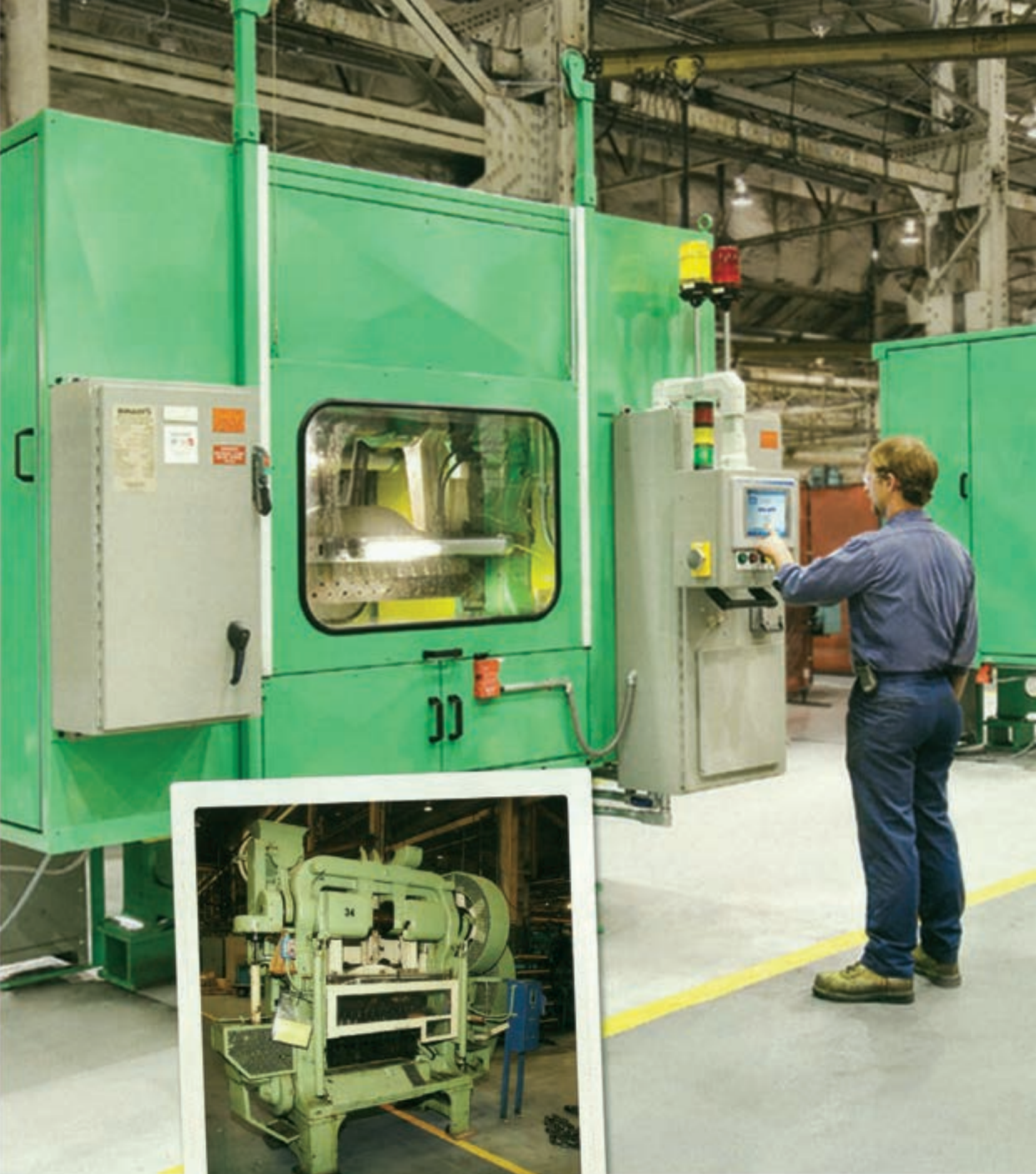
Bullet Assembly Machine (BAM) after rebuild with insulated sound enclosure and Allen Bradley PLC control.
